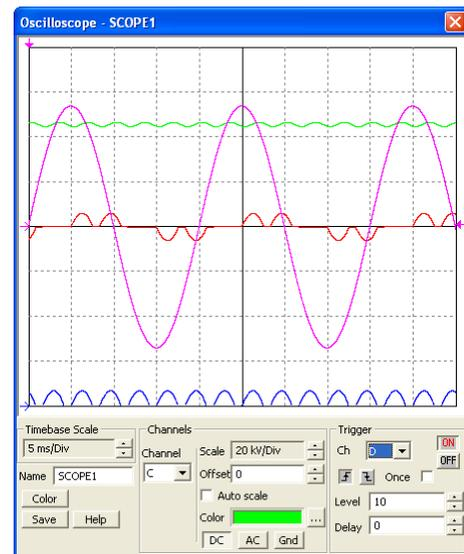
**Fig. 4 (b) Waveforms at low output ( $\alpha = 120^\circ$ )**
