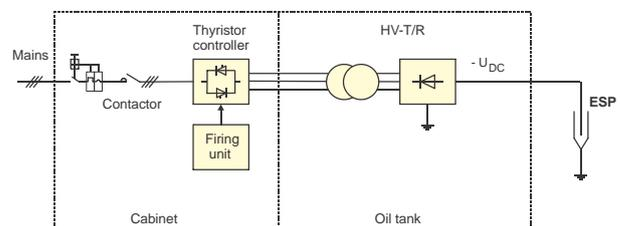
Fig. 1 Block diagram of a three-phase TR set
