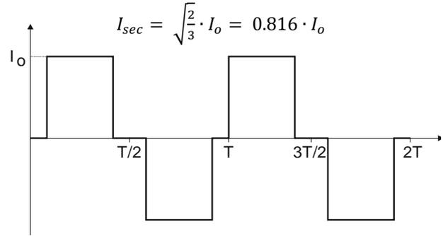
**Fig. 8** Ideal waveform of the current delivered by the secondary winding and its rms-value
