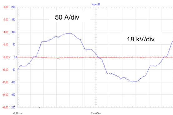
**Fig. 5 Primary current (blue) and ESP voltage (red) at rated current.**
