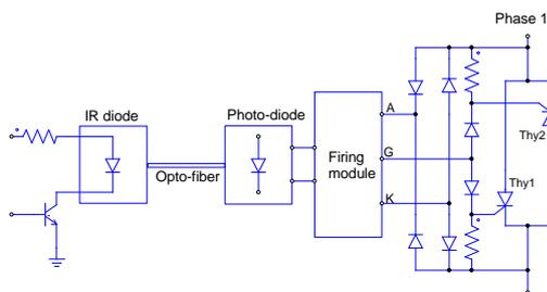
**Fig. 12 Solution with only one firing module per phase.**
