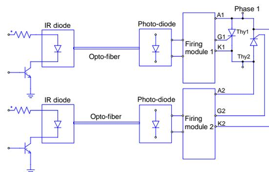
**Fig. 11 Solution with optical fibers**
