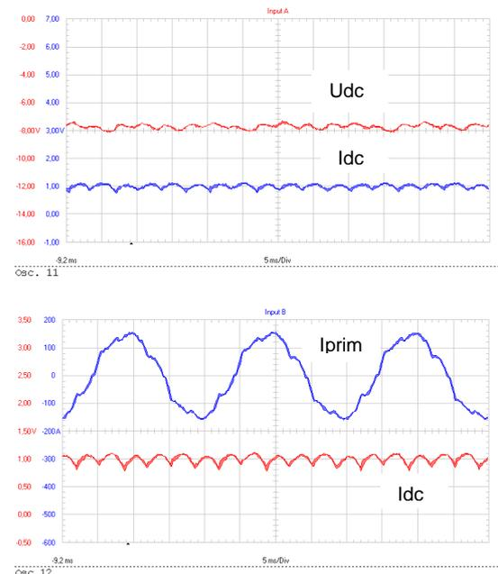
**Fig. 7 Main waveforms for a 1500 mA TR at rated ESP current.**
