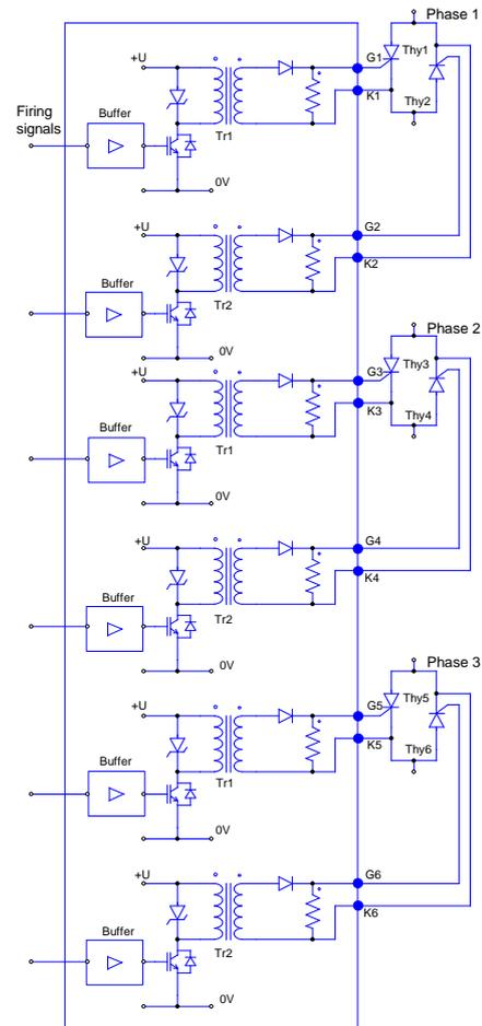
**Fig. 10 Traditional firing with 6 output stages.**
