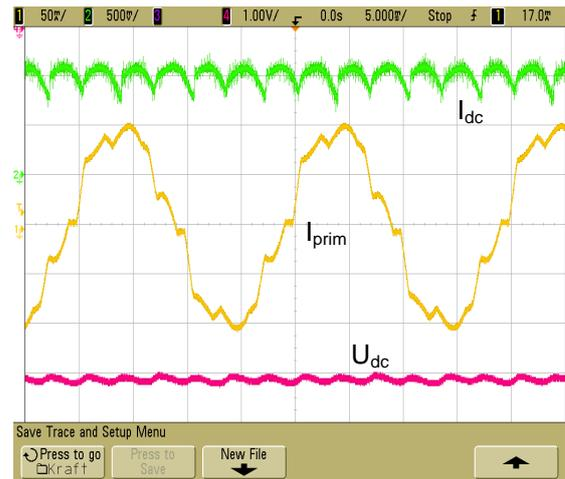
**Fig. 6 Primary current ( $I_{prim}$ ), ESP voltage ( $U_{dc}$ ) and ESP current ( $I_{dc}$ ) at rated value (600 mA).**
