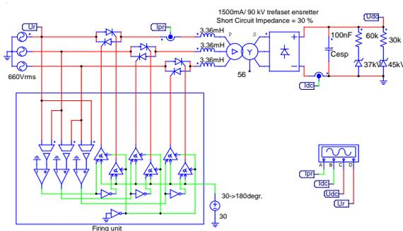
**Fig. 3 Simulation circuit of a 1500mA/90 kV three-phase TR set**
