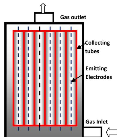
the steel frame and the steel frame was isolated / suspended through high voltage insulators. Water nozzles were provided through which water mist was generated and sprayed in the collecting electrodes tubes.
