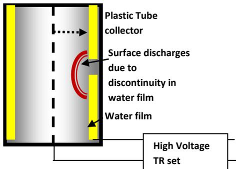
If the plastic tube part is not sufficiently wetted then there is discontinuity in the corona current path, creating surface discharges on the plastic tube collector. This reduces the effective voltage for collection and more dangerously, can seriously damage the plastic tube, because of the localized high temperature. If remain undetected /
