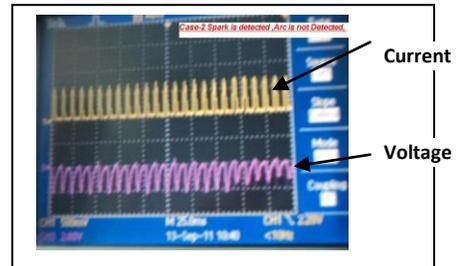
After carrying out various experiments with various conditions, a special algorithm was developed to sense such discharges. **This utilized the phase relation between primary current and input voltage. During surface discharges, the phase relation between primary current and input voltage changes and this change was additionally incorporated into the control system. This was an additional input to detect the surface discharges.**
