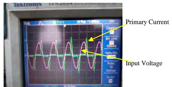
Various confirmatory tests were carried out to validate the algorithm, under various conditions. The surface discharges were detected and controlled. Typical output voltage and current waveforms as shown below;
