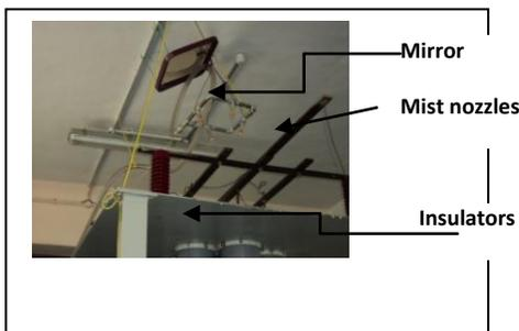
With moderate mist generation, the water film inside the plastic tube was adequate and continuous. In this condition, a voltage of approx. 35 KV with a current of about 50 mA was attained without any flashovers / discharges. After further increasing the voltage, normal flashovers occurred
