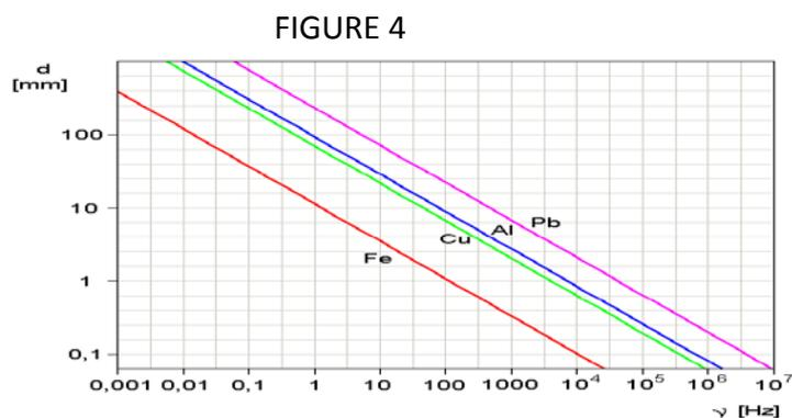
*Figure 4 shows the skin effect penetration for metals at differing frequencies.*
