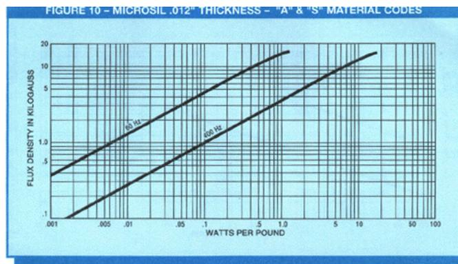
*Figure 3 above is a plot of core flux density vs. energy loss at 60Hz and 400 Hz. This chart from Magnetic Metals Corp publication.*
