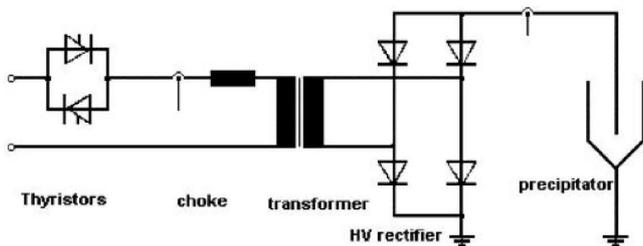
**Fig. 1.** Thyristor based HV power supply system for ESP [1] the voltage is quite high in Thyristor based power supplies which is around 30% of the peak. Since flashovers in precipitators usually occur close to the peak value of the precipitator voltage,  $V_{max}$  is limited by the Voltage
