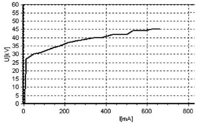
Fig. 9. Response of 50Hz supply system [4].
