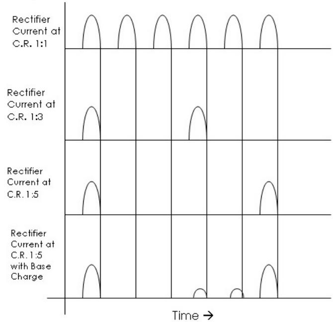
Fig. 6. Intermittent and base charge Control
