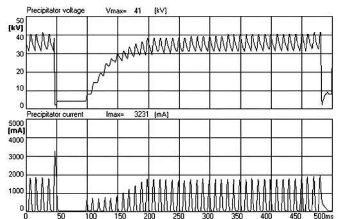
**Fig. 2.** Thyristor based Precipitator Voltage and Current [1]
