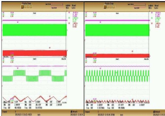
Fig. 15. No-load waveform @ fs = 6kHz, for F=50 & 500Hz.
