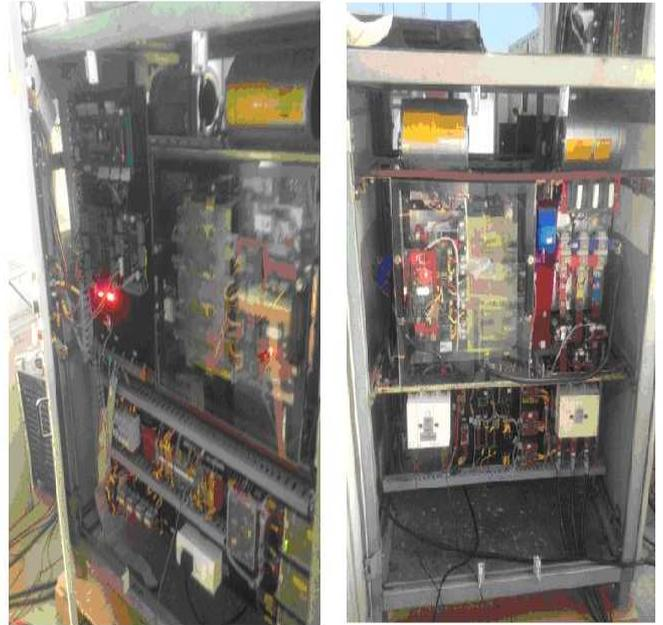
Fig. 14. Developed IGBT power supply system (front & back view)
