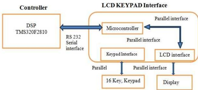
Fig. 8. Interface between DSP and Keypad/Display unit
