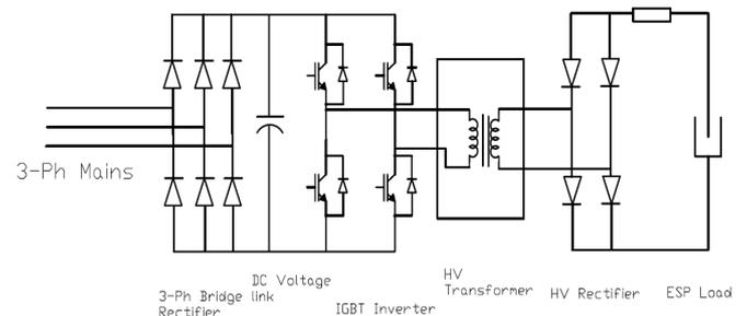
**Fig. 3.** Typical IGBT based HV power supply system
