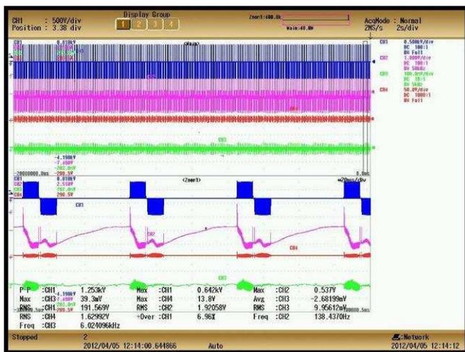
Fig. 17. Intermittent charging waveform with a charge ratio of 1:3.
