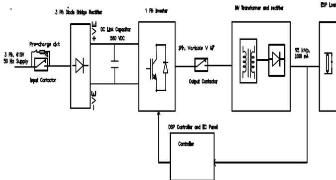
Fig. 4. Block diagram of the developed IGBT based HV power supply system
