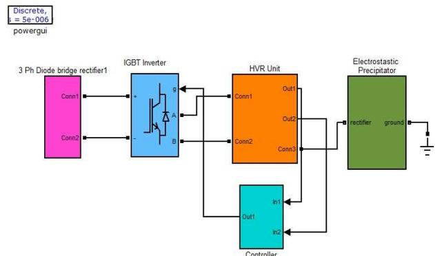
Fig. 10. Simulink model of IGBT based HV power supply
