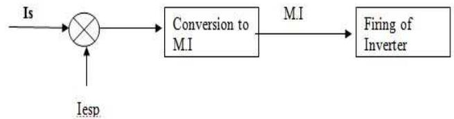
Fig. 5.  $I_s$  Control implementation in IGBT system
