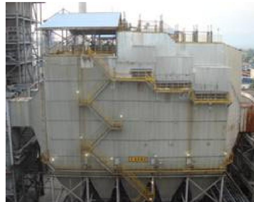
Figure 10 Reformed ESP-FF hybrid dust collector
