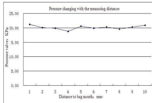
Fig11 Pressure drop distribution map of filter bags
