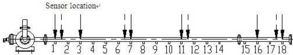
Fig4 Sketch map for the arrangement position of pressure sensor on jet pipe
