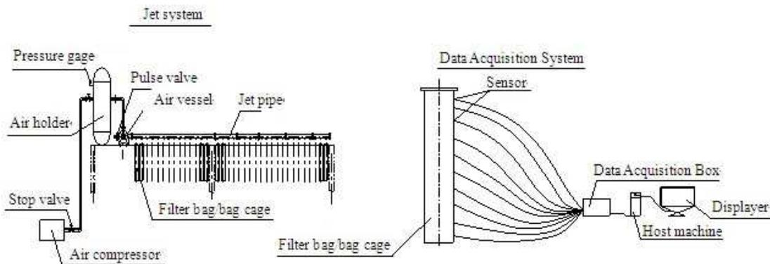
Fig 3 Jet system and data collection system
