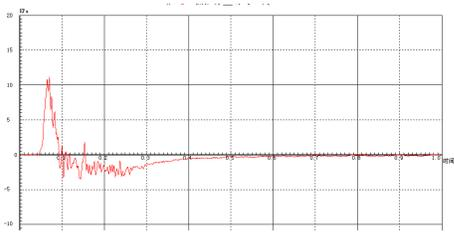
Fig7 Pressure drop changes with the time on the upper point (439 mm from the bag inlet)
