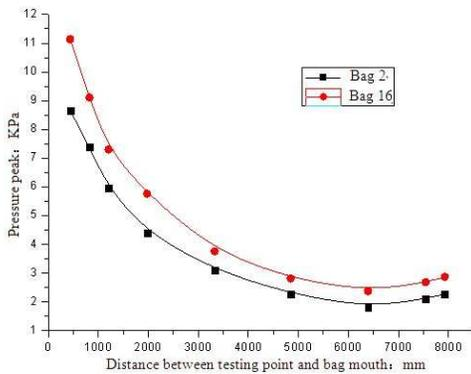
Fig10 Comparison of pressure drop distribution of no.2 and no.16 filter bags
