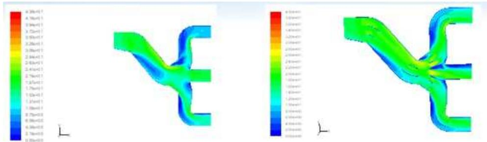
Fig12 Speed cloud picture without guide plates      Fig 13Speed cloud picture after guide plates installed
