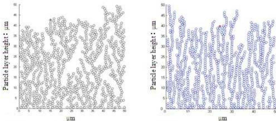
Fig17 Comparison chart for the arrangement of charged and uncharged dust particles (charged dust particles is on the right)
