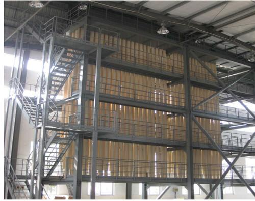
Fig2 Full-scale pulse jet experimental model
