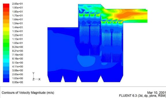
Fig14 Physical model of a 1000MW power unit; CFD model and velocity nephogram
