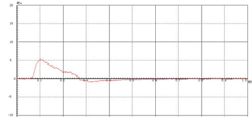
Fig8 Pressure drop changes with the time on the middle point (3327 mm from the bag inlet)
