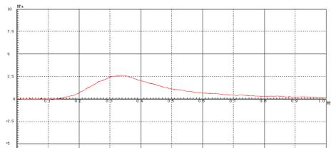
Fig9 Pressure drop changes with the time on the bottom point (7545 mm from the bag inlet)
